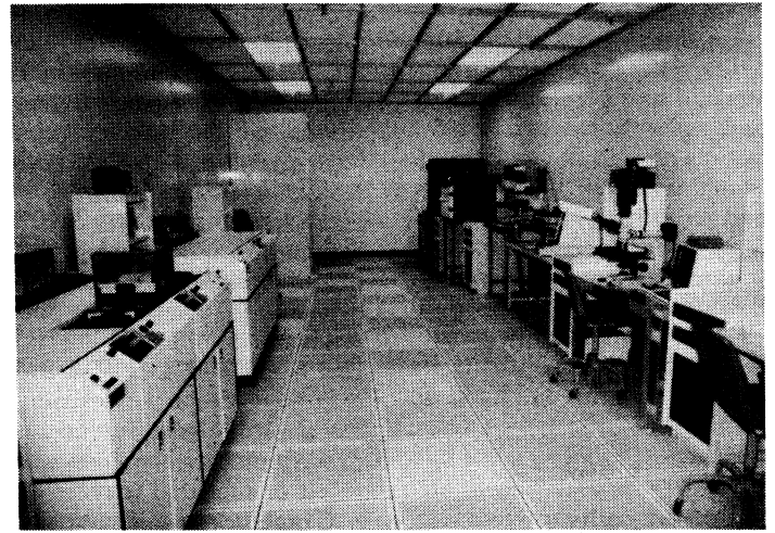
Photolithographic chamber where chips are exposed & etched.
